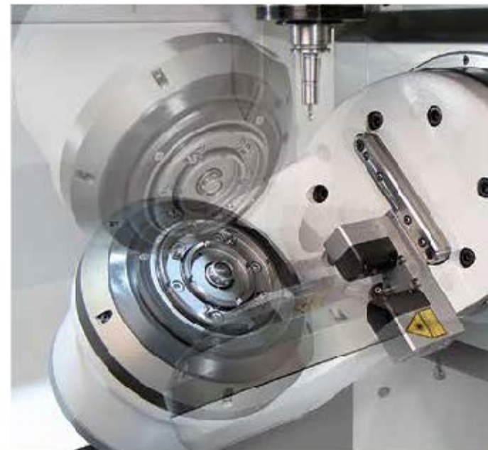
Pallet with coined cams
