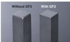
Electrode wear comparison for 0.6 x 0.6" and 1.6" depth
