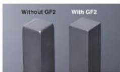
Electrode wear comparison for 0.6 x 0.6" and 1.6" depth
