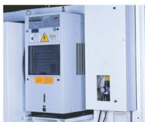
Spindle Oil Chiller
