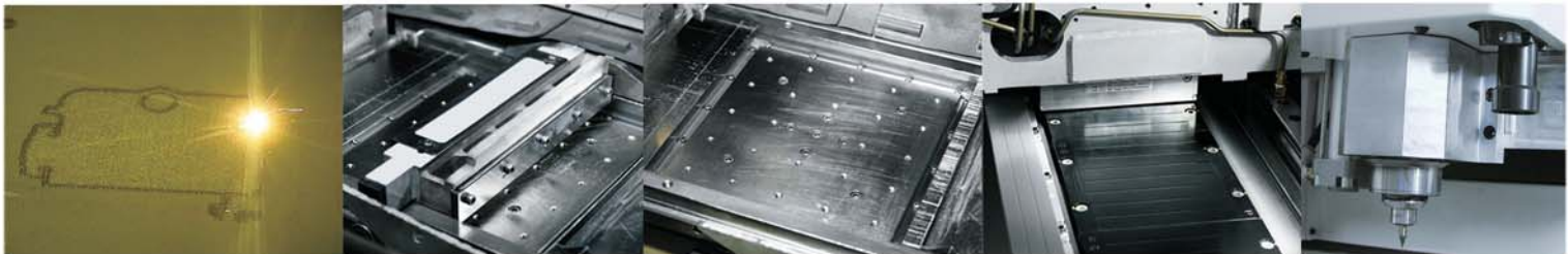
Yb 400w Fiber Laser uses Matsuura's Galvanometer Mirror to create the sintered profile
