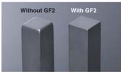
Electrode wear comparison for 0.6 x 0.6" and 1.6" depth
